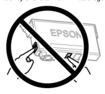
Do not touch the sections shown in the illustration of the cartridge.
