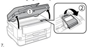
Raise the scanner unit and open the ink cartridge cover.
