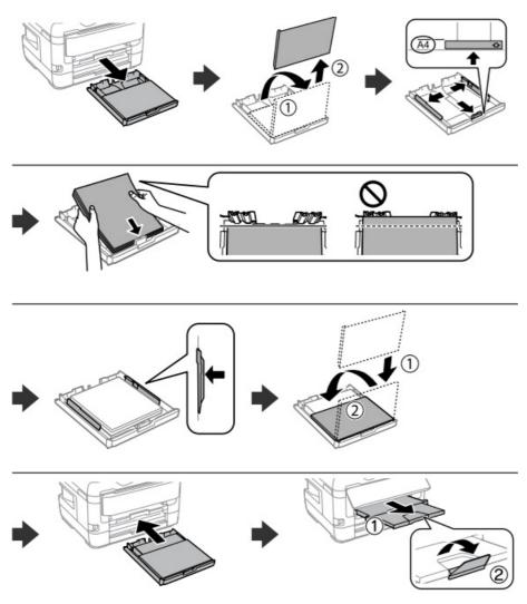
Load paper in the paper cassette with the printable side facing down. Do not load paper above the  $\bigvee$  arrow mark inside the edge guide.
