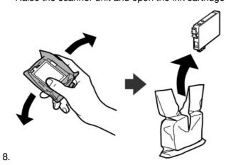
Gently shake all new ink cartridges four or five times and then remove it from its package.
