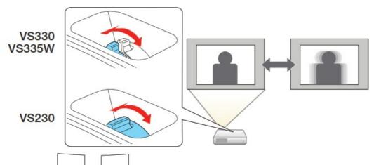
5. If your image looks like or you may have placed the projector off to one side of the screen at an angle. Place the projector directly in front of the center of the screen, facing the screen squarely. If you can't move the projector, use the horizontal keystone slider on the projector to correct the image.
