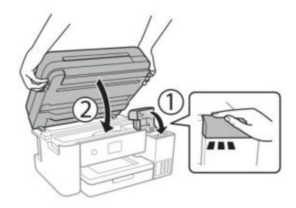
9. Raise the control panel, then press the  $\circlearrowleft$  power button to turn on the product. The  $\circlearrowleft$  power light flashes.
