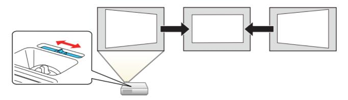
6. Your projector automatically adjusts images that look like or or, but if necessary you can press the button on the projector to correct it.
