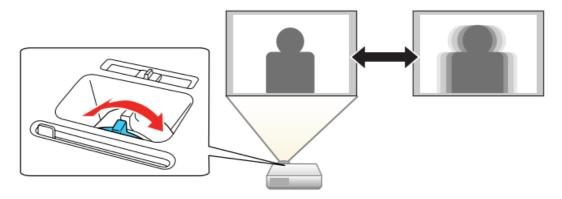
5. If your image looks like or or, you may have placed the projector off to one side of the screen at an angle. Place the projector directly in front of the center of the screen, facing the screen squarely. If you can't move the projector, use the horizontal keystone slider on the projector to correct the image shape.
