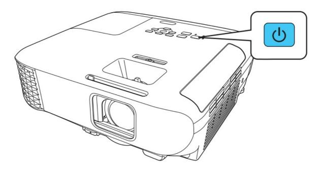
**Note:** To shut down the projector, press the opening power button twice.
