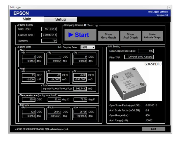
When "Show Attitude Graph" button is clicked, a plot graph of the attitude angle is displayed. On the Graph screen, measurements are expressed by numerical values and line graphs. In "IMU Display Select", select the IMU to display measurement values for. Push the close button (x) at the top right of the window to close the graph screen.
