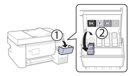
**Note:** Refer to the color-coded sticker above the ink tank unit to identify the color of each tank.
