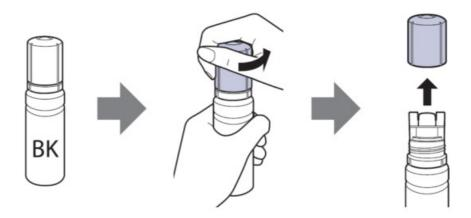
Caution: Do not shake or squeeze the ink bottle. Do not touch the top of the ink bottle after its cap is removed.
