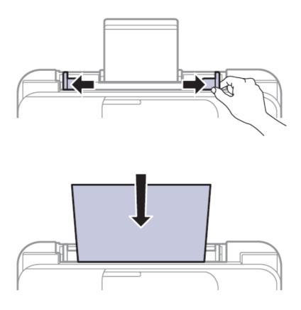
**Note:** Make sure the paper is under the mark inside the edge guides.
