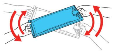
4. Match the color on the ink pack label with the color slot on the printer and then use both hands to insert the ink tray into the **printer.**
