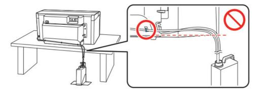
Note: Make sure the waste ink tube is not pinched anywhere or ink could leak inside or around the printer.
