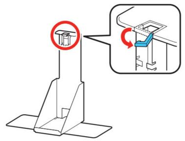
13. Place the tube next to the waste ink tube holder to check the length. Cut the tube about 0.4 inch (1 cm) below the bottom of the tube holder as shown.
