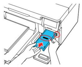
**Note:** The ink packs are keyed to fit into the correct color slot. If you cannot insert the ink tray all the way, do not force it. Make sure the ink pack color matches the color slot on the printer.
