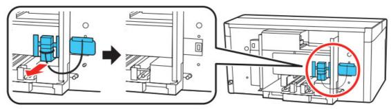
2. Holding a wipe to the waste ink outlets, remove the plugs on the back of the printer and then wipe the waste ink outlets as **shown.**
