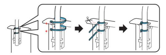
15. Insert the waste ink tube into the holder as shown and then close the clip.
