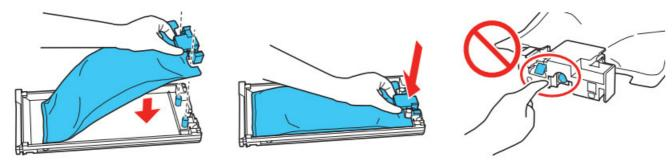
Note: Make sure the ink pack fits onto the pegs and is aligned with the top of the tray.
