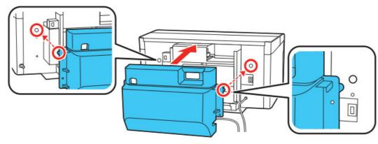
5. Tighten the rear cover screws.
