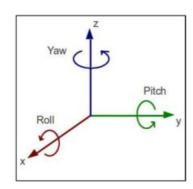
The projector can rotate around the 3 rotation axes:
