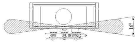
The rotation around this axis can be obtained: by turning the two front knobs in the same direction and by turning the rear one in the opposite direction. Also in this case, the rotation is  $\pm$ -8°.
