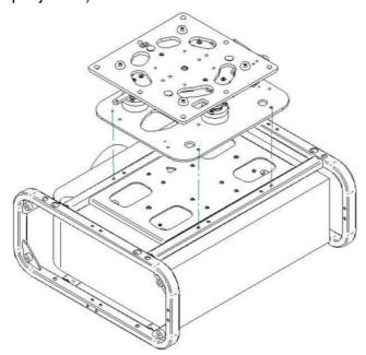
**NB:** The projector, screws and center distances indicated in the pictures above are merely an example for installation. Before mounting, it is necessary to check that the projector fastening positions are compatible with the KITE plate.
