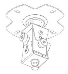
• Position the projector adaptor plate with adjustable arms on the bottom side of the projector.
