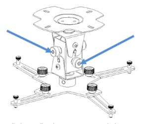
• Tighten the four button screws to eliminate vibration or movement during operation.
