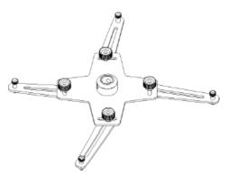
• Secure the adjustable arm plate to the projector by positioning the plate's screws with the designated holes on the bottom of the projector.
