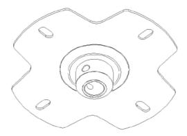
• Insert the calibration device into the ceiling plate
