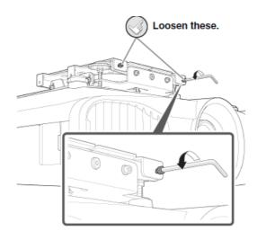
2. B While tightening the screws with the ball point hex wrench, fine tune the position.
