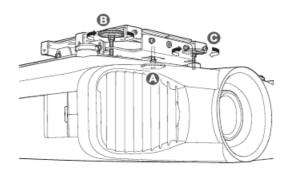
3. C After angle adjustment is complete, tighten the two screws firmly using the ball point hex wrench.
