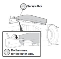
4. D Insert the M4x10 screws into the screw holes on the ceiling plate cover and tighten them with the ball point hex wrench.
