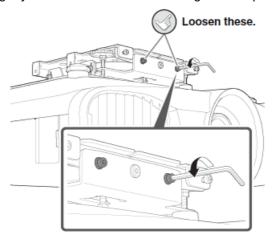
2. B Adjust the angle by turning the adjustment dial adjustment dial
