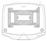
2. B Insert the M4x12 screws into the screw holes and tighten them with the Phillips screwdriver.
