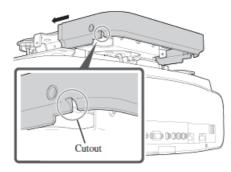
2. B Insert the M4x10 screws into the screw holes on the ceiling plate cover and tighten them with the ball point hex wrench.
