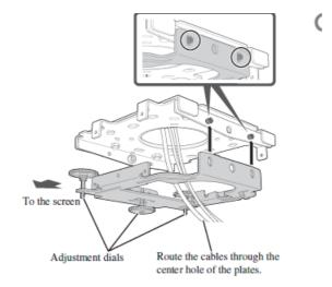
• B Insert the M8x10 screws into the screw holes on the ceiling plate and tighten them with the ball point hex wrench.
