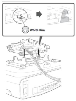
• B Slide the projector plate and engage the dowels on the projector plate into the cutouts on the ceiling plate .
