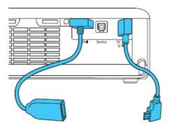
3. Connect the HDMI and USB cables to the streaming media player and fit it into the port compartment.
