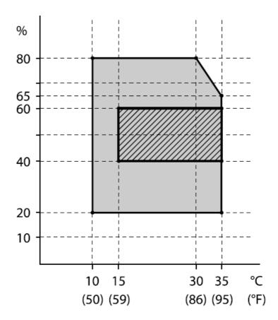
• Operating temperature and humidity (without condensation) range (the range shown by the darker rectangular area is recommended)
