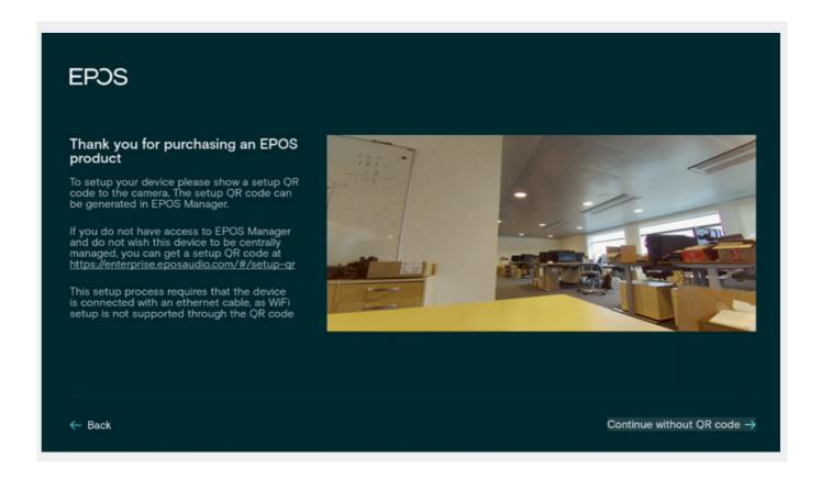
Use the created QR code to enroll the devices into EPOS Manager. The system will automatically deploy the settings contained in the QR code and upgrade the EXPAND Vision 5 and EXPAND Control to the latest FW.
