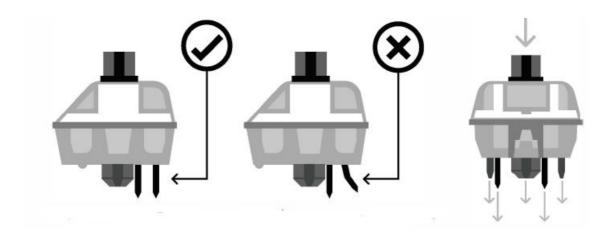
Before installing switches, be sure the pins are clean and straight.
