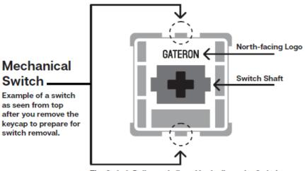
The Switch Puller tool aligns Vertically to the Switch to unclip the plastic securing the switch to the plate.
