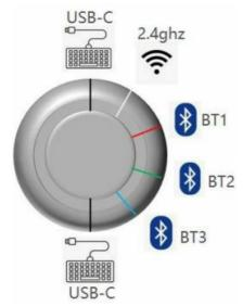
• **b**) The furthest you can rotate on both direction is for wired mode. And besides the two endpoint, you can rotate the knob clock wise for 2.4ghz wireless, Bluetooth 1, 2 and 3.
