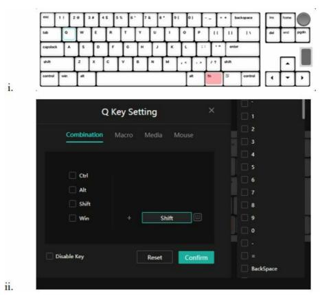
• c) Use FN+Z/X/C to toggle between the 3 layouts. And you can check out which key layout you have activated with the screen.
