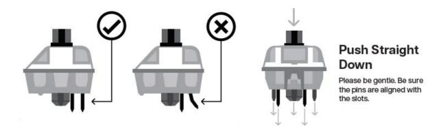
Before installing switches, be sure the pins are clean and straight.
