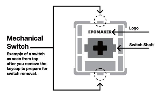
• The Switch Puller tool aligns Vertically to the Switch to unclip the plastic securing the switch to the plate.
