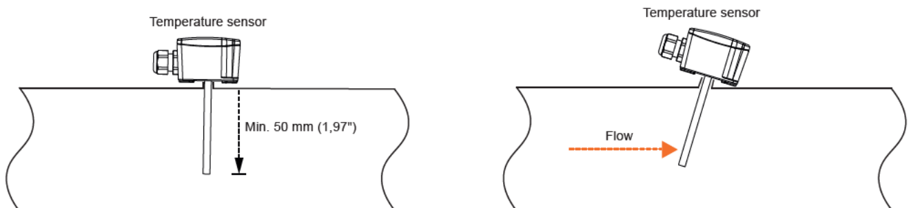
Fig. 4 Correct position in a pipe
