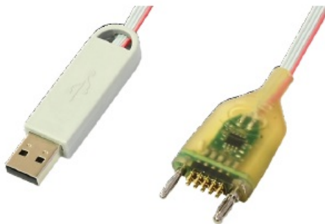
Fig. 7 HA011023 USB Configuration Adapter for EE431 with analogue output
