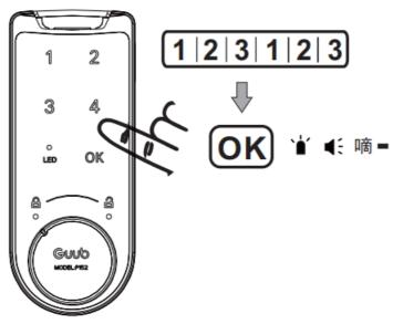
2. Turn the knob to "a" position then unlock successfully
