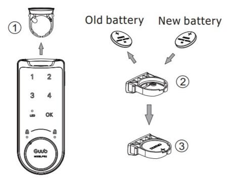
Notice: Positive of battery should be up position
