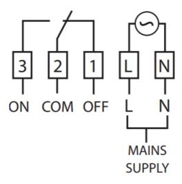
• If the mains voltage output is required, terminals L & 2 must be electrically linked.
