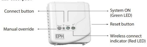
**Wireless connect:** Once voltage has been applied this button may be pressed to initialise the pairing process with the wireless thermostat.
