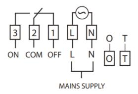
\* If mains voltage output is required, terminals L & 2 must be electrically linked. **Important**: Do not connect Mains Voltage to OpenTherm® terminals.
