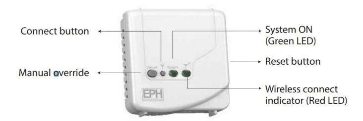
Wireless connect: Once voltage has been applied this button may be pressed to initialise the pairing process with the wireless thermostat. Once pressed the red LED will begin to flash.
