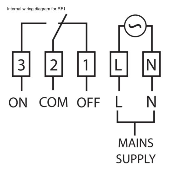
If mains voltage output is required, terminals L & 2 must be electrically linked.
