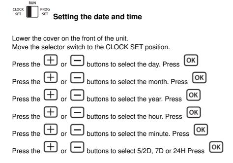
The date, time and function are now set. Move the selector switch to the RUN position to run the program, or to the PROG SET position to change the program setting.
