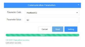
1. Select a communication parameter from the [Parameter Code] drop-down list and click the "Read" button to read the parameter.
