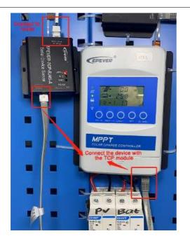
1. Connect the TCP module's "COM" port or RS485 i nterface with the device. The detailed communication cable refers to chapter 1.2 Applicable products. And connect the TCP module's "Ethernet" port to the router by a network cable (The TCP module and the PC must share the same network).
