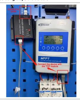
1. Connect the TCP module's "COM" port or RS485 interface with the device. The d etailed communication cable refers to cha pter 1.2 Applicable products. And connect the TCP module's "Ethernet" port to the ro uter by a network cable (The TCP module and the PC must share the same network).
