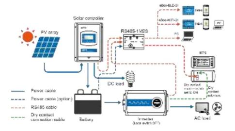
**Note:** When the power consumption of the external monitoring device is large, an external power connected to the auxiliary port can be used to power the device.
