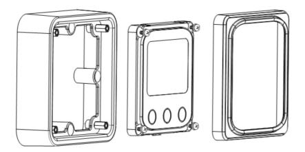
**Step1:** Locate and drill screw holes based on the Frame Mounting dimension of the base, and erect the plastic expansion bolts.
