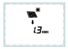
Press the and button and hold on 5s to clear the generated energy.
