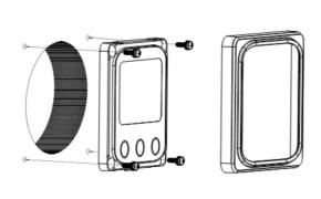
**Step1:** Locate and drill screw holes based on the installation size of the surface.
