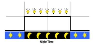
Turn-On voltage (Adjustable): 5V(12Vsystem), delay10min. Turn-Off voltage (Adjustable): 6V(12Vsystem), delay10min. Note: 24V system voltage×2
