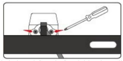
3. Position the license plate bracket onto the license plate, line up the holes and secure with screws.
