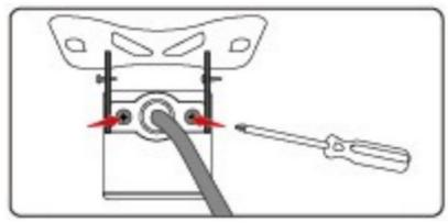
2. Install the camera to the license plate bracket and secure with the screws.
