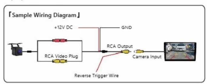
**Note:** This wiring diagram is just for reference. Please seek assistance from professionals for different situations. **Note:** If the voltage/current of the reverse lamp of some cars (especially made by VW Group) is unstable, it is recommended to use BATT or ACC with relay.
