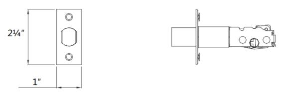
Adjustment instruction of deadbolt. When adjusting, rotate the "deadbolt" (as the picture).
