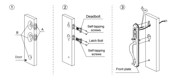
1. Make holes in door "A" and "B" at 2-1/8", and for the Grip Handl e bottom screw (per template).
