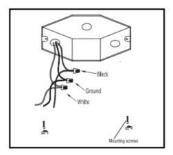
1. Turn OFF/disconnect power at circuit breaker. Typical junction box wiring has only white and black switched wires controlled by wall switch for ON/OFF or dimming. Ensure the junction box has an additional set of unswitched wires (continuous) main power wires as shown.
