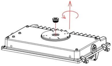
6. According to the embedded terminal box, punch the corresponding mounting hole on the light's mount.
