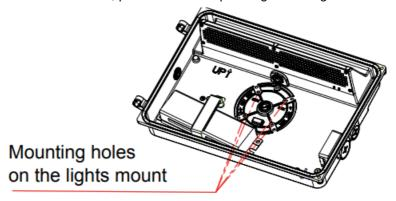
7. Put the input line in the embedded box through the waterproof pad and then pass through the lamp base.
