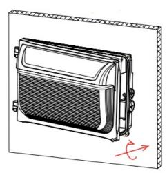
13. Fill the gap between the lamp and the wall with silicone sealant to prevent rainwater from entering the junction
