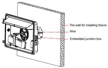
8. Use a screw to lock the lamp base on the embedded junction box and ensure the balance of the horizontal column.
