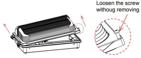
5. Unscrew the cover of the entry hole on the lamp base and remove the cover.
