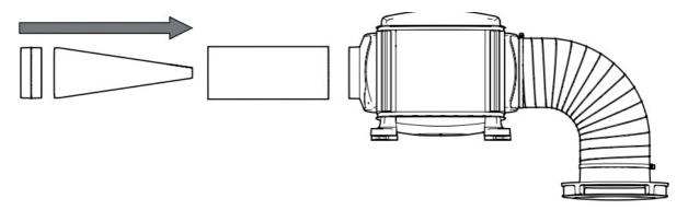
• Connect to the filter with a section of flexible duct approximately 300mm long (not supplied). The connection must be removable, to allow the filter to be replaced. Connect this to an external vent (see page 5 for examples).
