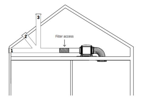
Use one of three options to connect the inline duct to the outside of the property (extra parts not supplied):
