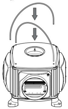
• Insert the two flexible filter rods into the holes in the lid so they cross in the middle.
