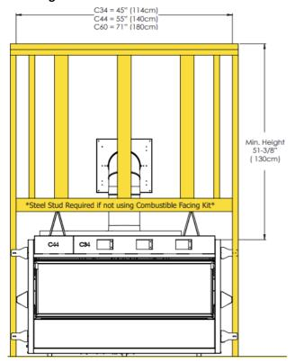
CSS Side Vent (Horizontal Install) - Min. Framing & Clearances
