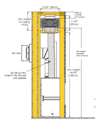
\*NOTE: 15.75" from the header is required for min. ceiling height. Rest unit on lower standoff. There will be a 3/4" (2cm) gap on from the top standoff to the header in this configuration.
