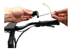
• Step 4: With this bolt removed, the hinge at the bottom will open.
