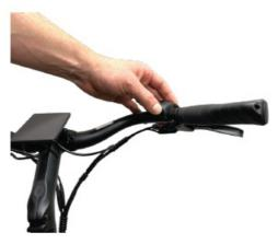
• Step 6: Insert the hex bolt removed in Step 3 and rotate clockwise until the controller is snug, but not fully tight.
