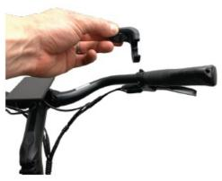
• Step 5: Place the handlebar controller on the bicycle handlebar.
