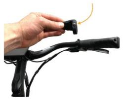
• Step 3: Rotate counterclockwise until it is fully removed – do not lose this bolt.
