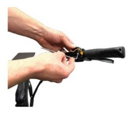
• Step 7: Rotate the controller on the handlebar and adjust for a comfortable position to press the buttons while riding. This can be adjusted again at a later time. Use the hex wrench to fully tighten the handlebar controller so it does not move while riding.
