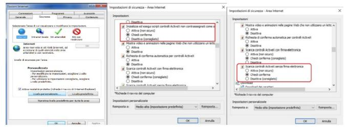
In the Internet Explorer address bar, enter the IP address of the camera <a href="http://192.168.1.10">http://192.168.1.10</a> Select "Allow", when Internet Explorer asks for permission to install ActiveX controls
