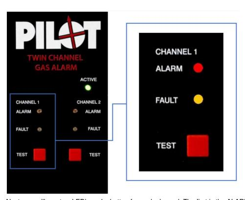
Next, you will see two LED's and a button for each channel. The first is the ALARM LED and will illuminate red
