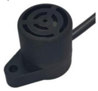
The LPG sensors detect butane/propane and alarms at 25% LEL (lower explosive limit). LPG gases are heavier than air, therefore the LPG sensor must be located near to the floor.
