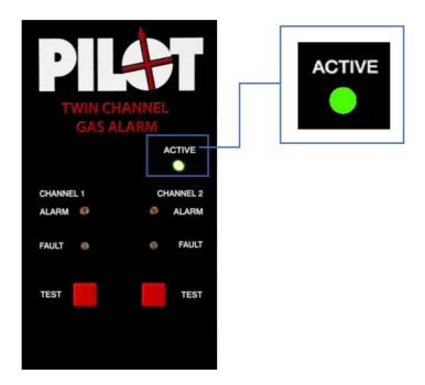
The first LED on the front panel of your Twin Channel Gas Alarm is the Power Indicator. This LED illuminates green when the unit is powered on.
