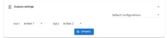
Drop-down in the upper right corner allows to set all outputs to one protocol with one click.
