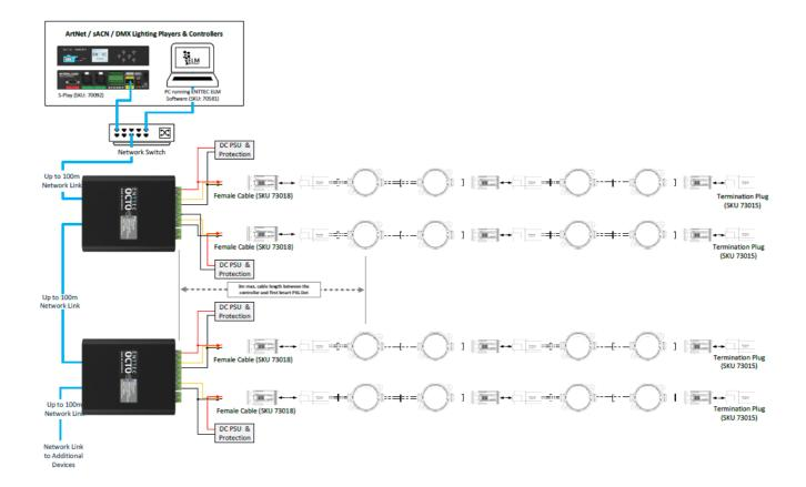
Note: If the power or data source to your controller drops out whilst the Smart PXL Dots remain powered, the last state will be held until either the data feed resumes or power to the Smart PXL Dots is disconnected and re-connected.
