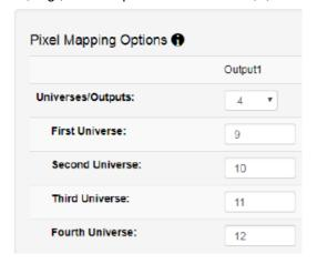
Each output can also be specified to use its own individual group of universes, e.g., output 1 uses universes 100,101,102 and 103 however output 2 uses 1,2,3 and 4.
