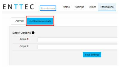
Standalone is to be used to create a looping effect that can be played back from the point the OCTO is powered on. – This can also be of use to test the OCTO's output without the need to send eDMX data. Standalone can be activated by clicking on the 'Use Standalone mode' button as shown below: When activated, the word Standalone will be displayed next to the ENTTEC logo.
