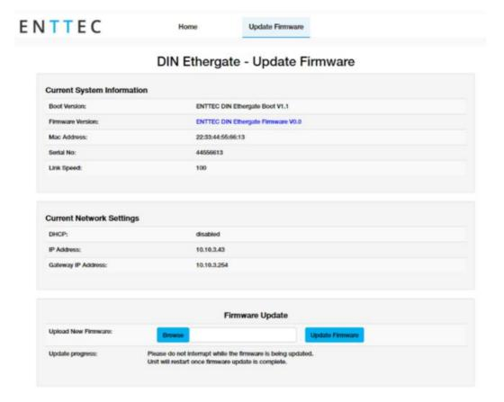
After the update has been completed, the web interface will load the Home tab, where you can check if the update was successful under Firmware Version. Once the Home tab has loaded, the DIN ETHERGATE will resume operation.
