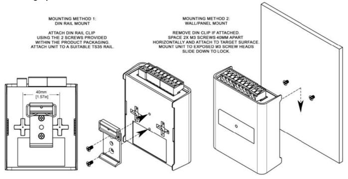
**Note:** The surface mount tabs have been designed to hold the weight of the OCTO MK2 only, excess force by cable strain can cause damage.
