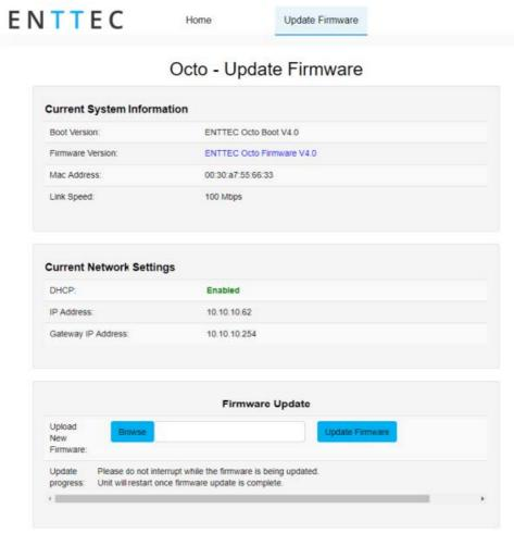
When selecting the Update Firmware tab, the OCTO MK2 will stop outputting and the web interface boots into the Update Firmware mode. It may take a while depending on the network setting.
