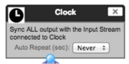
**Clock:** Allows you to synchronize ALL Pixel Link output only when the connected Input Stream is received. The Clock module can be used to make sure the output is always synced to the "latest universe" especially if the source adds a delay to each universe.
