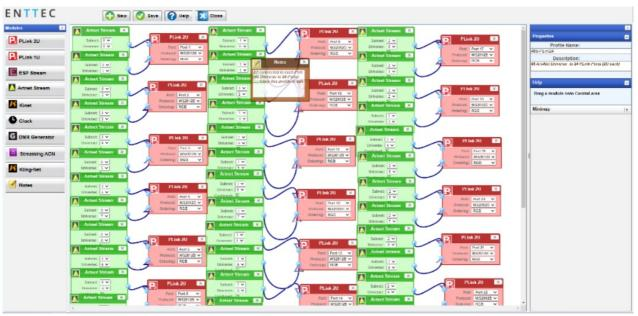
The direction of the wire (arrow) is important, the arrow signifies output, and reflects the flow of data. The same PLINK port# cannot be re-used within the same profile.
