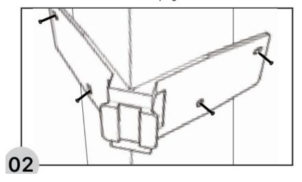
3. Buckle the motion light and the mounting plate to the brackets securely
