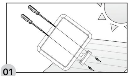
2. Use a power drill (not included) to dri the holes on your chosen wall perpendicular corner. Place the brack plate over the holes & use the include wall plugs and screws to fasten the bracket plate to the surface
