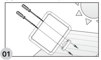
2. Use a power drill (not included) to drill the holes on your chosen mounting surface Place the mounting plate (with smooth surface facing out) over the holes & use 2 of the included wall plugs and screws to fasten the mounting blate to the surface
