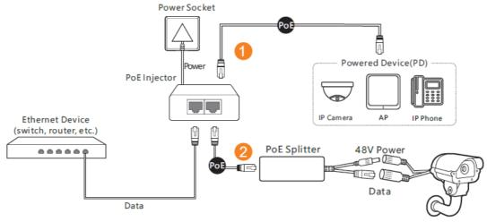
Method 2: The PoE injector and PoE splitter work as a kit to supply 48V power and transmit data to a device which does not support PoE function.
