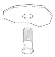
**Step 4:** Thread the plain end of the nut from behind the tile to secure the carrier. If the tile is thicker than normal, flip the nut and thread the ribbed end of the nut to secure the carrier.
