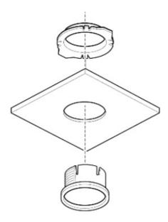
**Step 5:** Slide the tabs of the nut along the keys of the carrier to fasten the carrier.
