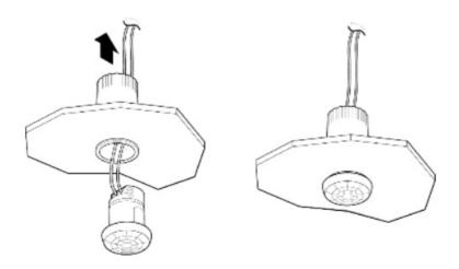
**Step 8:** Leave four inches of slack cable in the sequence loop to avoid pinching of the cable and to bring the sensor down if it needs to be replaced.
