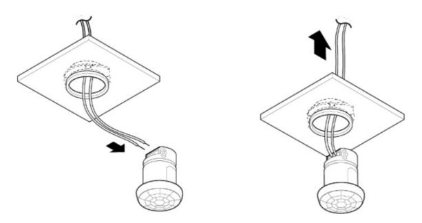
**Step 7:** Insert one end of the pair of wires through the hole in the fixture and connect the wires to the sensor.
