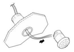
**Step 7:** Guiding the wire from above, push the sensor into the carrier until it securely clicks into the carrier.
