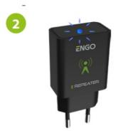
Make sure the repeater is connected to power supply. The blue LED should flash.
