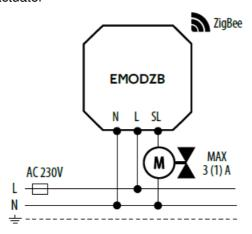
• b) Connection diagram to the control box
