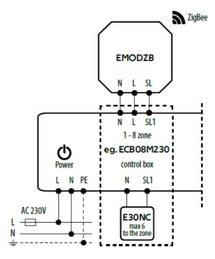
• c) Connection diagram as a ZigBee repeater
