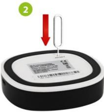
Make sure the gateway is powered on. Using the PIN included, press and hold the RESET button for 8 seconds until LEDs start lighting up. The pairing mode is enabled.
